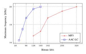
Figure 9: Frequency bandwidth of MP3 and AAC.
