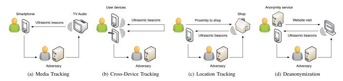
Figure 1: Examples of different privacy threats introduced by ultrasonic side channels. (a) Ultrasonic beacons are embedded in TV audio to track the viewing habits of a user; (b) ultrasonic beacons are used to track a user across multiple devices; (c) the user's location is precisely tracked inside a store using ultrasonic signals; (d) visitors of a website are de-anonymized through ultrasonic beacons sent by the website.
