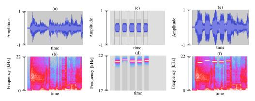
Figure 5: Example of transmission of ultrasonic beacons. The upper three panels depict the audio wave of an audio signal, while the lower three panels show the corresponding Spectrogram. (a)-(b) show a music track, (c)-(d) an ultrasonic beacon, (e)-(f) show the result after embedding the beacon into the original track.
