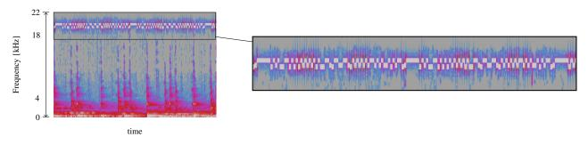
Figure 6: Spectrogram of a disclosed Lisnr audio beacon. An FSK scheme encodes a repeating bit sequence in the near-ultrasonic frequency range between 18.5 and 19.5 kHz.
